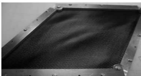
FIG. 9. Wrinkling phenomenon observed at 40° shearing angle on the carbon fabric.
