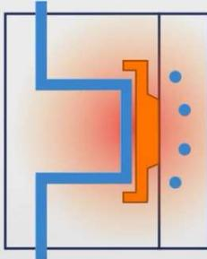
The part reheats the cavity, improving the next injection phase
