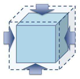
> Warpage -> Change of shape of the part during solidification and cooling phase, due to various physical phenomena interacting in a very complex way (uneven packing, uneven cooling, uneven shrinkage, anisotropic material properties, ...)
