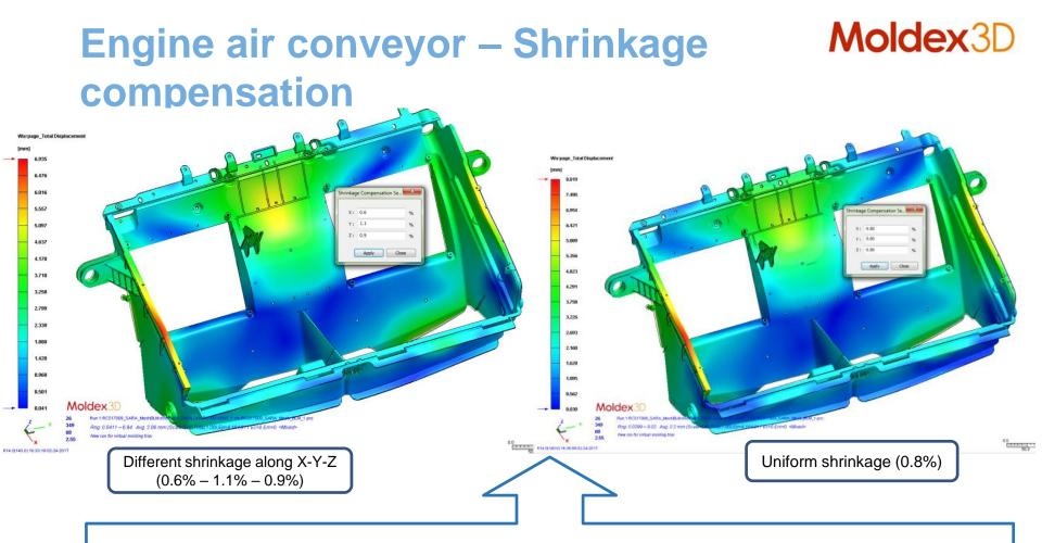
Tentative to find out the **optimal value** of nominal linear shrinkage to apply in toolmaking. MOLDEX allows to **compensate warpage from shrinkage effect by setting a custom X,Y,Z %** value.
