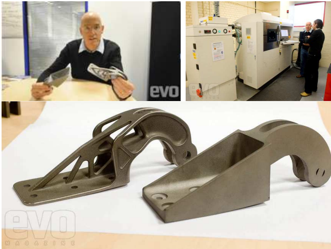
Door bracket for A380 – DML and Conventional EOS Ti64 produced on EOSINT M 270Xt at EADS IW.
